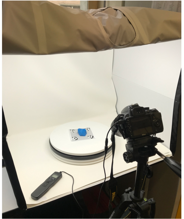
Fig. 2. Example of the setup used to acquire the images by using a photographic tent and a Nikon D3100. The image shows the camera, the turntable, the 3D-STD placed on a rectangular scale and the remote camera control which is used to avoid any image movement.
