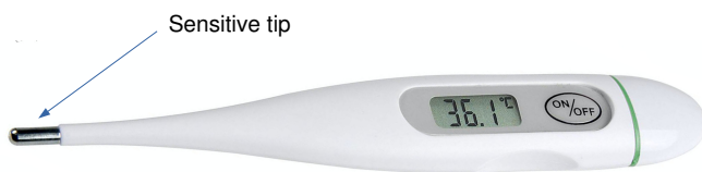
Fig. 7. A contact electronic thermometer, similar to the mercury thermometer.
