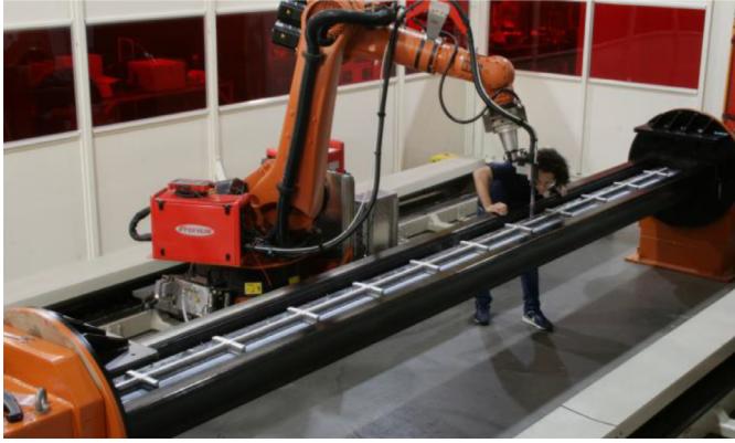
Fig. 1. Overall view of the WAAM system (Cranfield University).
