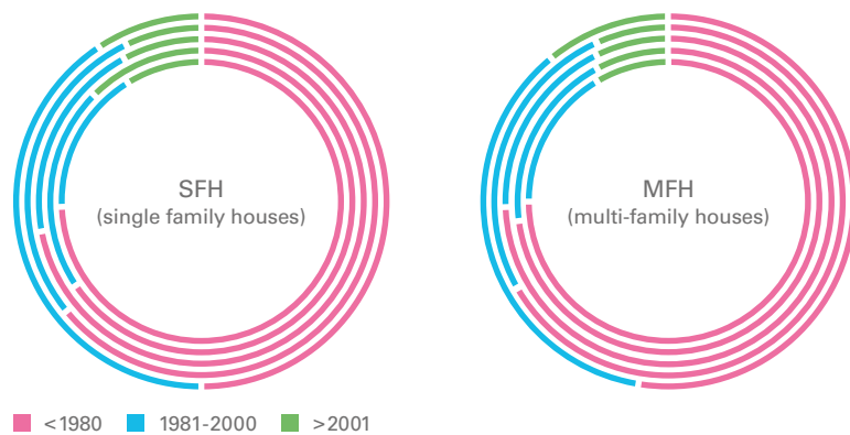
Figure 7 Distribution of residential buildings per typological class and geographical zone (from innermost to outermost circle: North-west, North-east, Center, South and Islands areas). Elaboration on [2] and [11].
