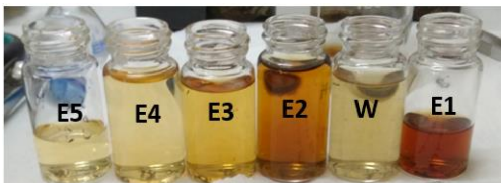
Figure 31. Washing treatment of a spent catalyst after APR of hydrolysate 0.9 wt.% C at 270 °C.
