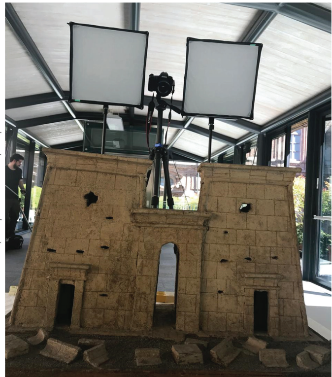
Fig.4 - Strategy of acquisition through circles with four different assets (left): in blue images alignment and in the middle the SfM based tie-points extraction. Positioning of the maquette and photogrammetric set (right)
