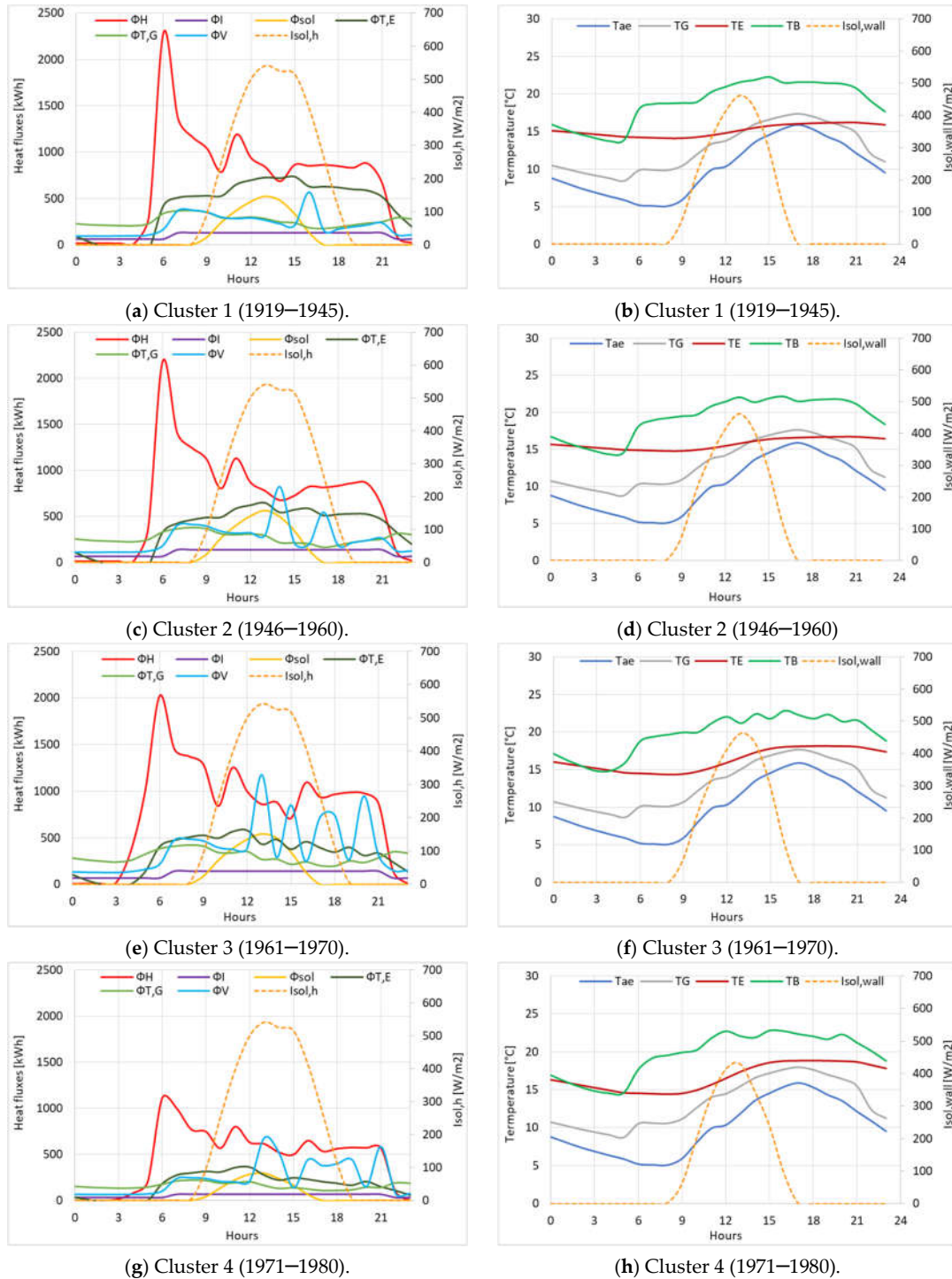
Figure 8. Heat flux components and building temperatures (with a variable number of air changes per hour and windows opening) for a typical day: February 22 nd 2014, with a T_{ac}=6.24 °C (clusters for the four construction periods).
