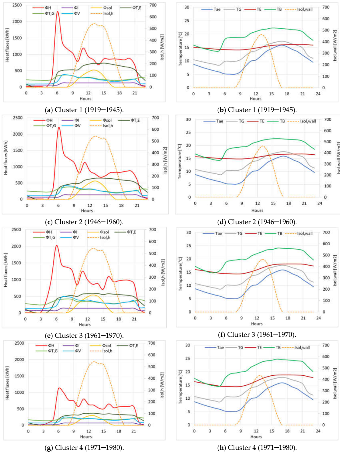
Figure 7. Heat flux components and building temperatures with a variable number of air changes per hour (in daytime ach = 0.62 \text{ h}^{-1} , and in nighttime ach = 0.3 \text{ h}^{-1} ) for a typical day: February 22 nd 2014, with a T_{ae} = 6.24 \text{ °C} (clusters for the four construction periods).
