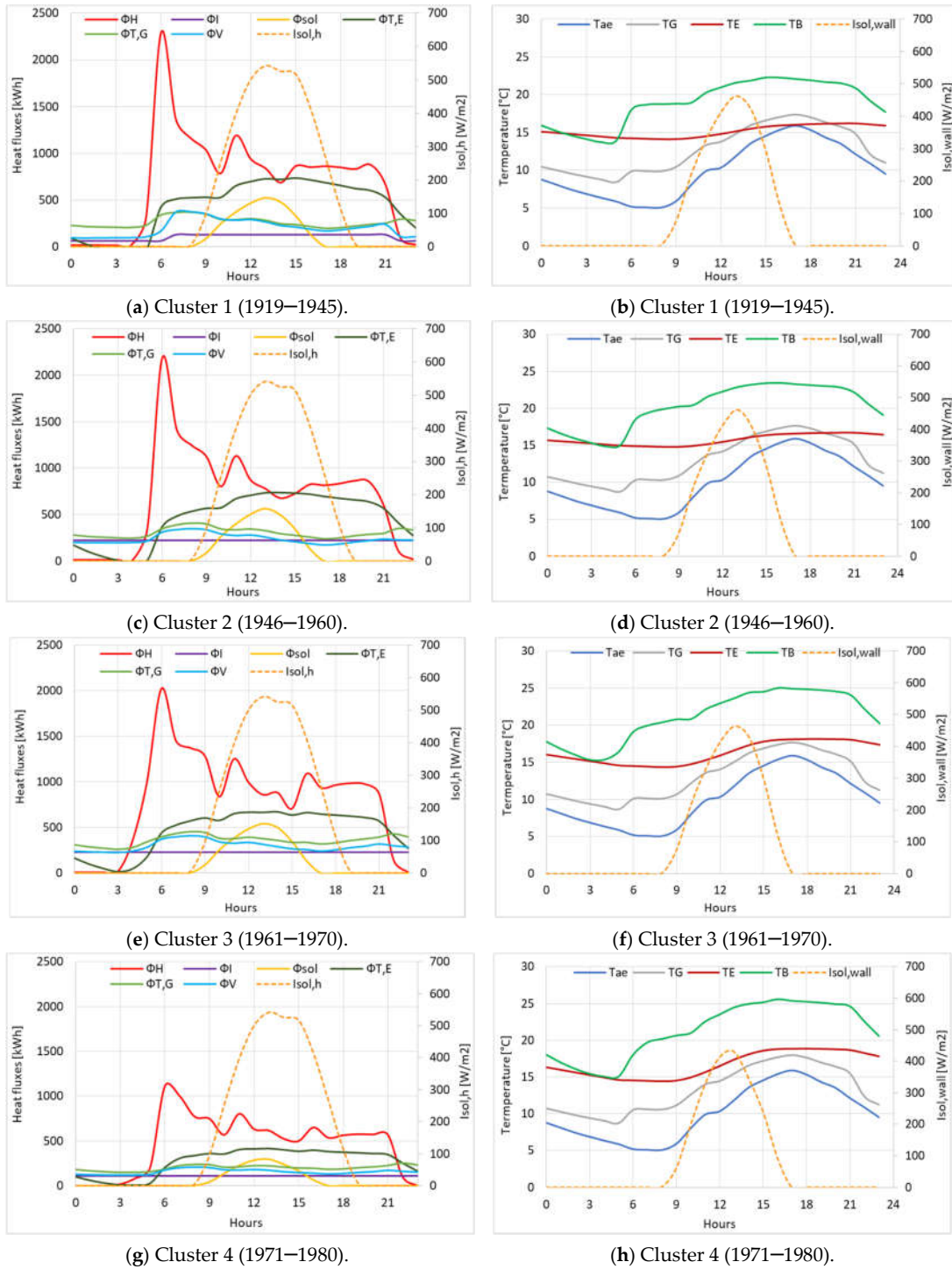
Figure 6. Heat flux components and building temperatures (with constant ach = 0.5 h -1 ) for a typical day: February 22 nd 2014, with a T_{ac} = 6.24 °C (clusters for the four construction periods).
