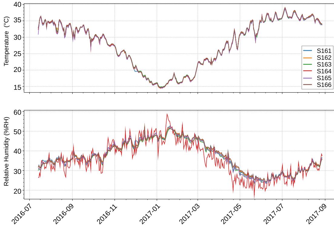
Fig. 4. T and RH measurements collected for one year during the Sohag Museum monitoring campaign from the smart sensors inside (S161, S162, S163, S165, S166) and outside (S164) the showcases.
