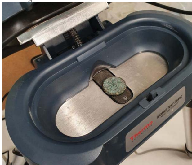
Fig. 3. Coin positioned for pXRF analysis.
