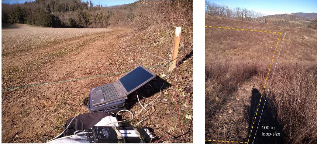
Figure 5.20 Some pictures of the TDEM survey carried out around Travale in February 2019 (left) the instrument used for TDEM acquisition was a TEMFAST48; (right) the most accessible sites allowed a loop-size of 100 m to be set up.
