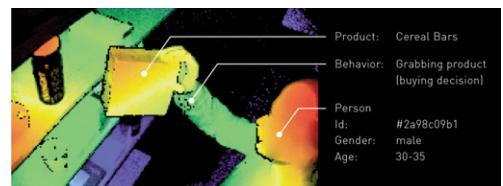
**Fig. 9, 10** | AI-powered Xovis 3D sensors detect when a person takes an article from a shelf (source: [www.xovis.com](http://www.xovis.com)).
