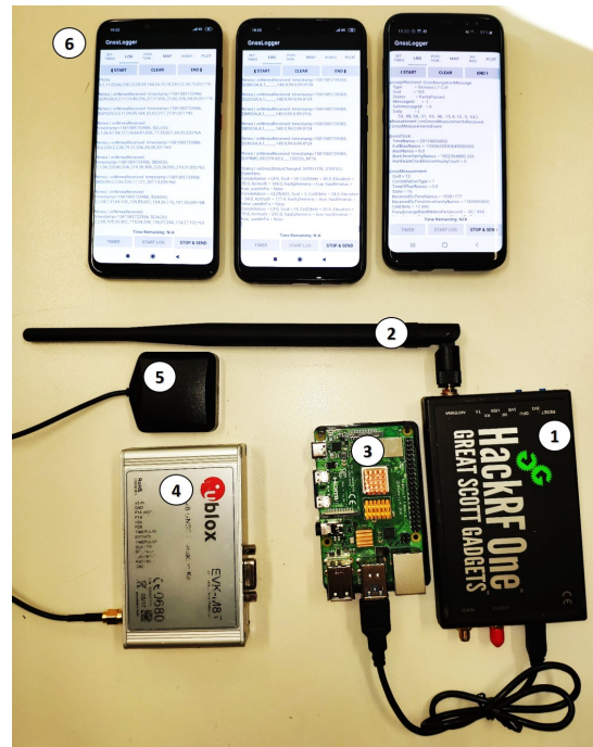
Fig. 2. Experimental setup consisting of a HackRF One, (1) equipped with an L1 stick antenna, (2), a Raspberry Pi 4B, (3) a u-blox™ Neo-M8N GNSS, (4) with an active GNSS antenna, (5) and a set of smartphones, (6) listed in Table I.
