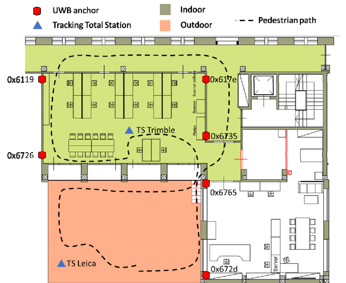
Fig. 2. The pedestrian path, the UWB anchor location and the indoor/outdoor spaces.
