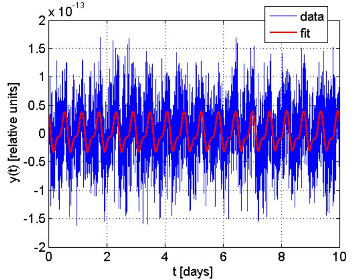
Fig. 3. Fit of the two periodic signals corresponding to the first two harmonics (peaks) of the power spectrum (red curve), along with the drift-removed fractional frequency deviation (blue curve).
