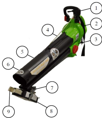
Fig. 5. The portable device for detaching and harvesting Crocus Sativus flowers on fields
