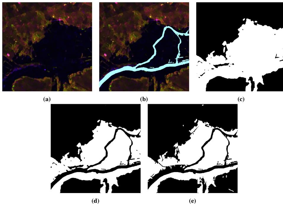
**Figure 2.** Example of performance improvement with the addition of hydrography layer for EMSRI49 - 13PORTUMNA, U-Net results: (a) Denoised input without hydrography, (b) Denoised input with hydrography, (c) Classification without hydrography (F1-Score = 89,2%), (d) Classification with hydrography (F1-Score = 96,8%), (e) Ground truth.
