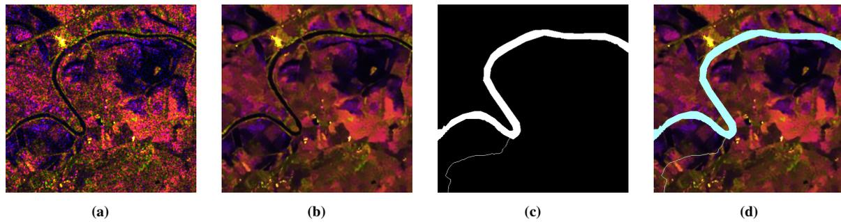
**Figure 1.** Pre-processing operations steps: (a) RGB Ratio, (b) RGB Ratio + Non Local Mean, (c) Hydrography Layer, (d) RGB Ratio + Non Local Mean + Hydrography.
