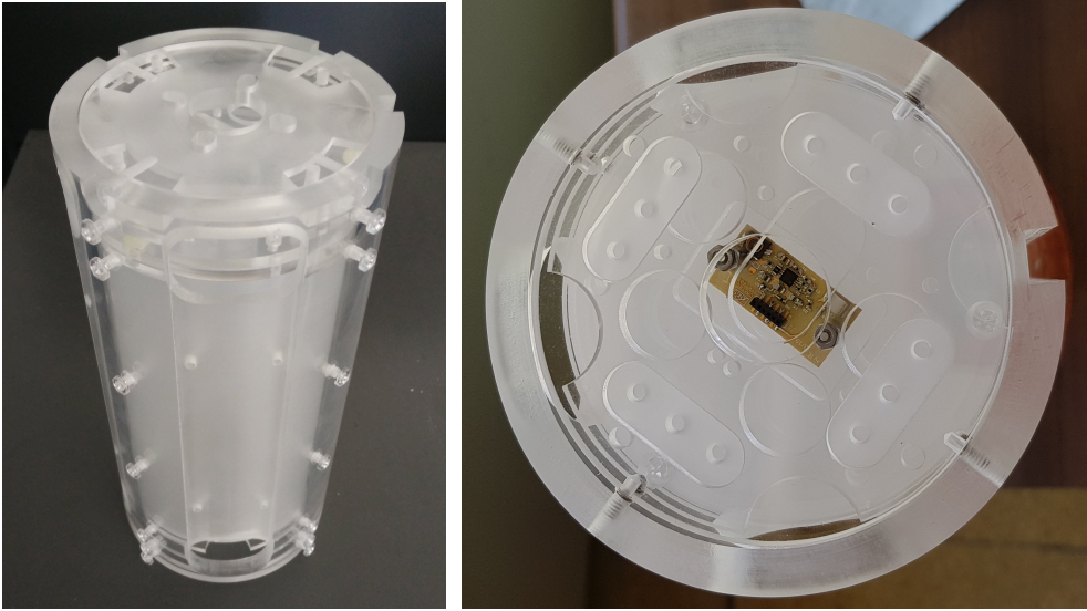
Figure 3. (Left) Inner acrylic structure lateral view. (Right) Top acrylic cap and support disk with the photo-detector module installed.
