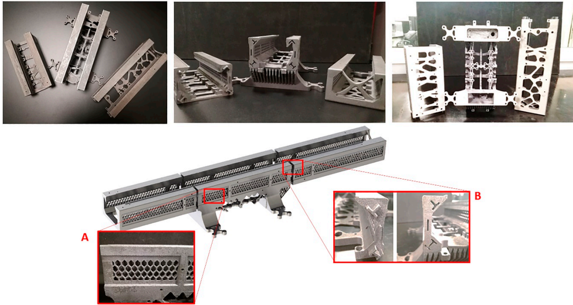
Figure 8. Technical prototype with details of the walls of the X-rail (A) and the shaft-hub interference fit (B).
