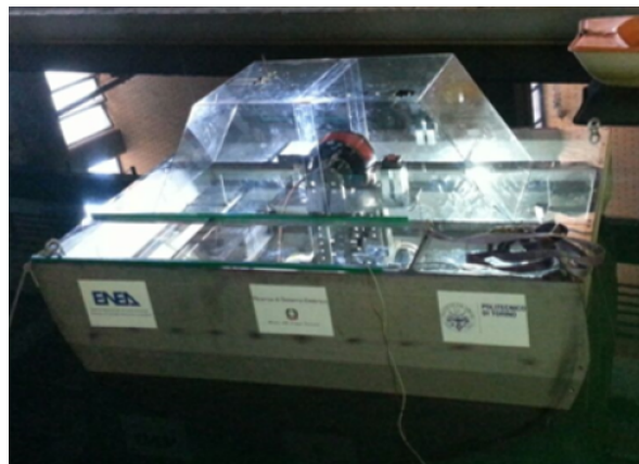
Figure 3. Photo of the 1:12 PeWEC prototype tested a wave tank [31].
