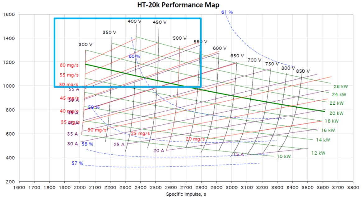
**Figure 3: Hall Effect Thrusters Functional Map (credits: SITAEL). The data range used in the simulation is highlighted in the blue box. the points in the database are specified by the intersections between the power (kW) and the voltage (V).**
