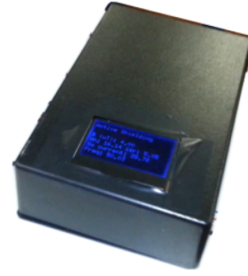
Fig. 1: Prototype of the active shield controller
