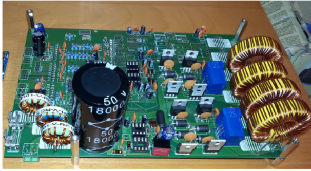
Fig. 1: Prototype of the active shield controller
