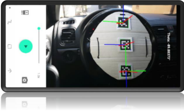
Figure 5. Markers detection through the rear-facing camera.
