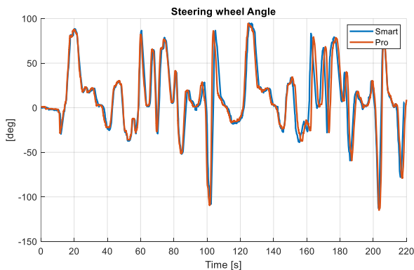
Figure 14 – Experimental validation: steering wheel angle during a lap on the handling test track.
