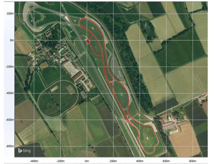
Figure 8. Top view of the handling test track. The red line is the car trajectory during a lap.
