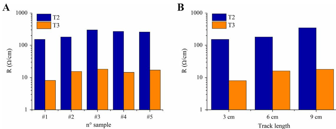
**Fig. 10.** Electrical resistance (logarithmic scale) of tracks treated according to T2 and T3 laser parameters: (A) reproducibility between different plates and (B) resistance of track with different length (3, 6 and 12 cm).
