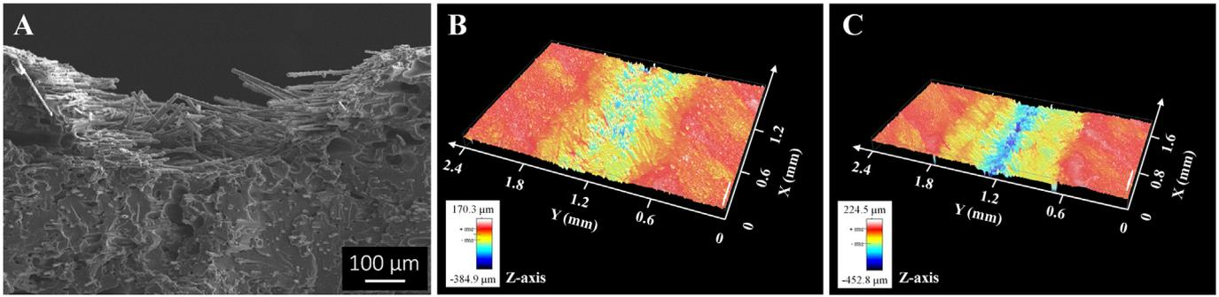
**Fig. 9.** (A) FESEM micrographs showing the cross section of the track obtained with T2 set of parameters and (B,C) surface topography (3D micrographs) of two conductive tracks printed with different laser parameters: (B) T2 and (C) T3. The colour map shows the depth of the track along the z-axis.
