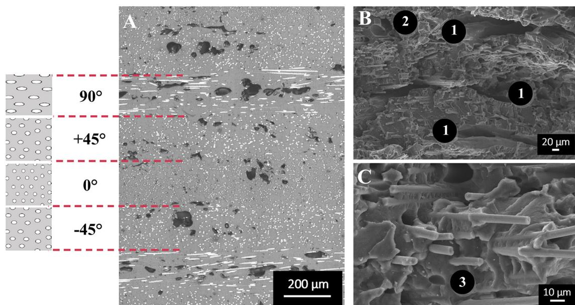
**Fig. 5.** (A) Optical micrograph of the polished surface of dog-bone cross-section printed with [+45, 0, -45, 90] architecture and (B,C) FESEM micrographs of the fracture surface of tensile samples printed at [±45°]. In fig. (A) the cross sections of the fibers observed within the layers are schematically sketched. In (B) different type of voids are highlighted: (1) inter-bead voids, (2) inner-beads voids and (3) cavity caused by fiber pull-out.
