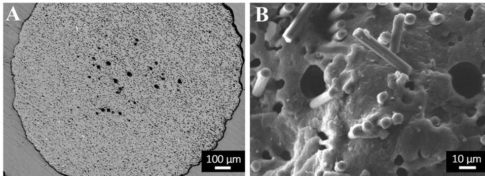
**Fig. 3.** (A) Optical micrograph of the polished filament cross-section and (B) FESEM micrograph of the cryogenically fractured filament, showing pores and carbon fibers aligned in the extrusion direction.
