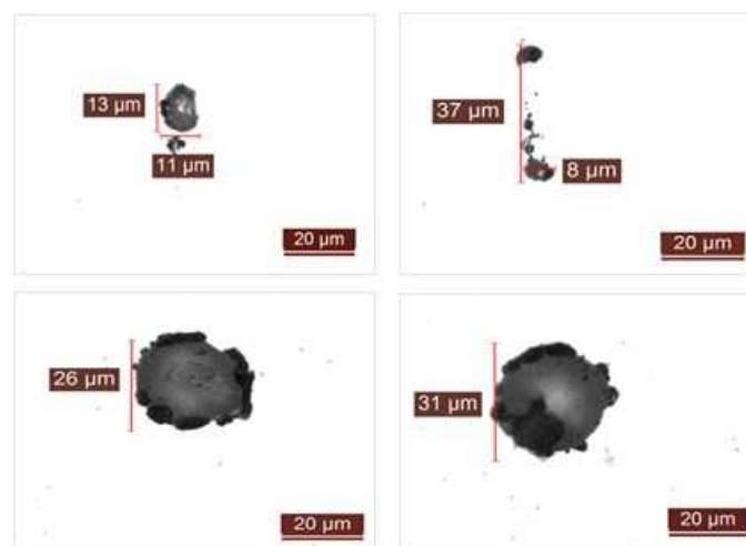
Fig. 2 - Oxides type - 1000x. Grade A (top) and Grade B (down)
