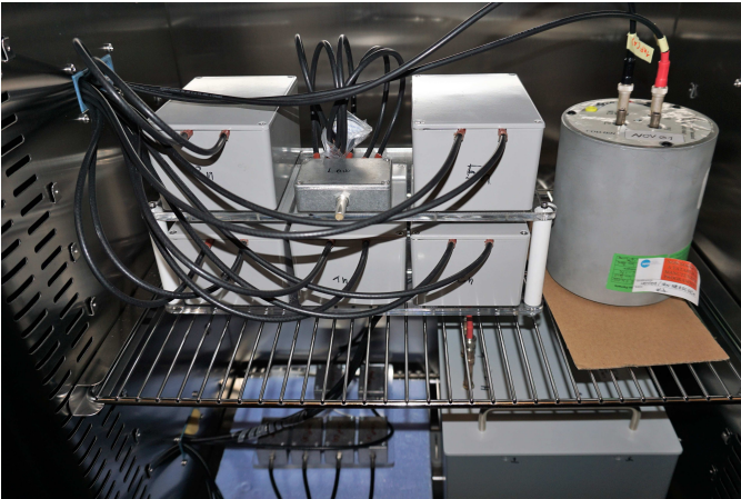
Fig. 2: Photograph of the base capacitors used in the experiment in the range from 1 nF to 10 nF. The capacitors are individually shielded and placed inside a thermostatic chamber.
