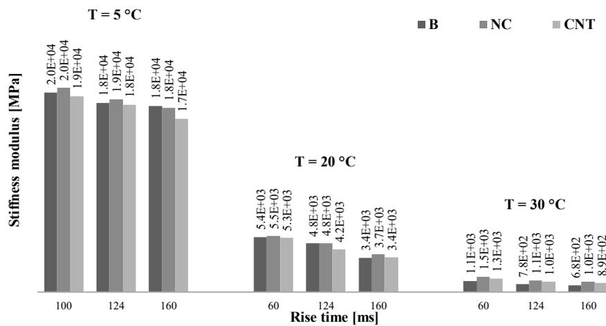
Fig. 2 Stiffness moduli of asphalt mixtures
