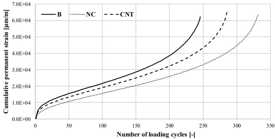
**Fig. 3** Typical curves obtained in flow number tests
