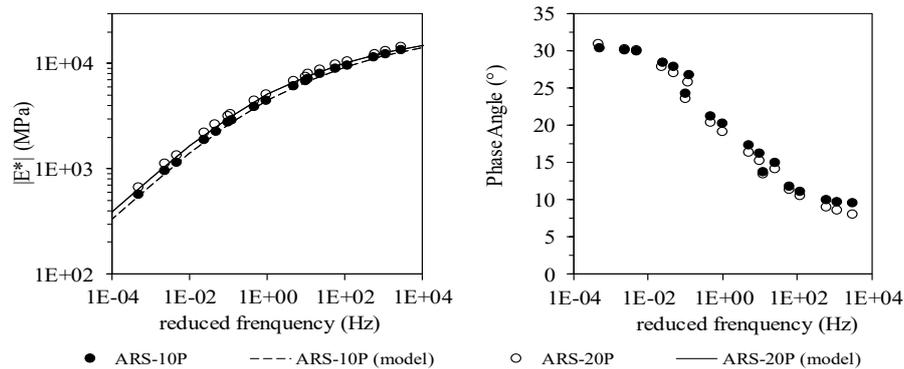
**Fig. 3** Master curves of mixtures ARS-10P and ARS-20P
