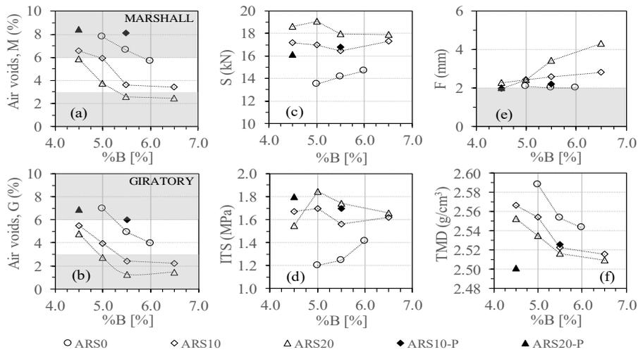
**Fig. 2** Mix design and quality assurance results: Marshall air voids content (a), gyratory air voids content (b), Marshall stability, S (c), ITS (d), Marshall flow, F (e), and theoretical maximum density, TMD (f)
