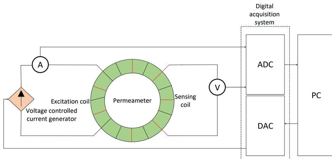
Figure 2. Measurement system layout.
