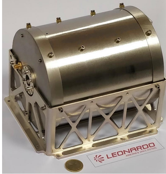
Figure 5.2: Picture of the realized engineering model EM1. Dimensions 35\text{ cm} \times 24\text{ cm} \times 20\text{ cm} . Total mass \simeq 3\text{ kg} . Courtesy of Leonardo S.p.A.
