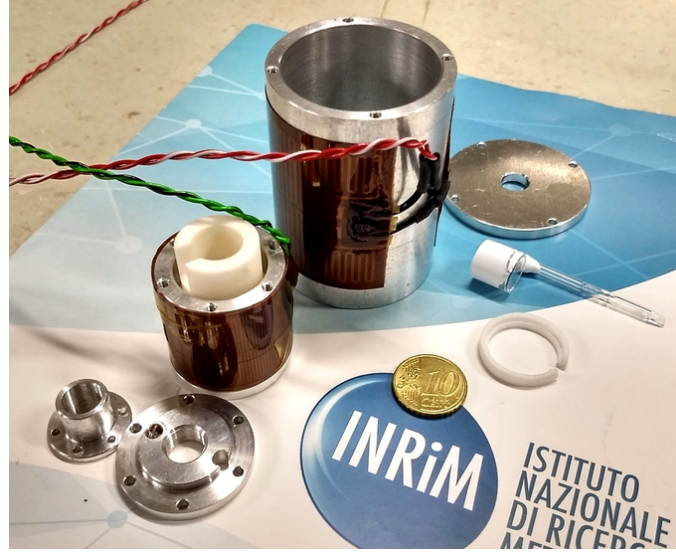
Figure 4.10: Picture of the building components of the cavity cell assembly. As a dimensional reference, a 10-cent of euro coin is shown.
