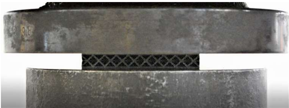
Figure 4.4: Zwick Roell machine setup for uniaxial compression test on a Octet-truss sandwich panel.
