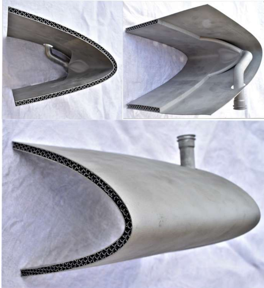
Figure 4.82: Mock-up of the anti-ice system designed for Piaggio P180 aircraft and produced with L-PBF.
