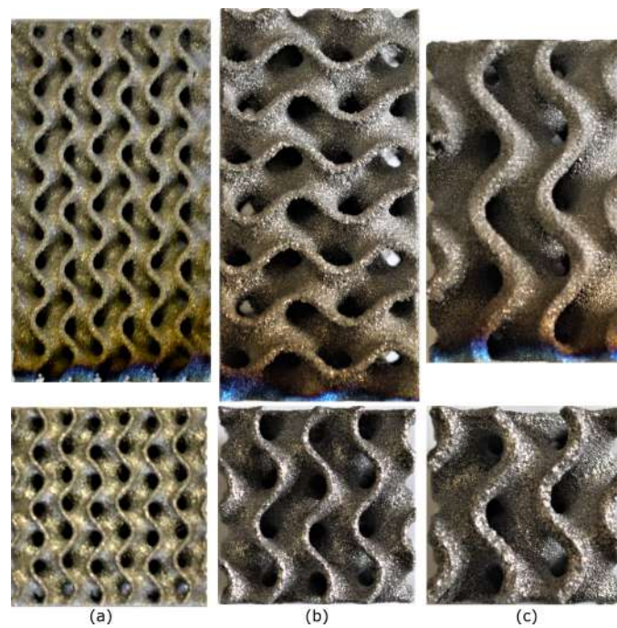
Figure B.17: Lateral and top view of the Gyroid Ti6Al4V specimens: a) Gyr-3-30-13, b) Gyr-5-25-1 and c) Gyr-7-35-1.
