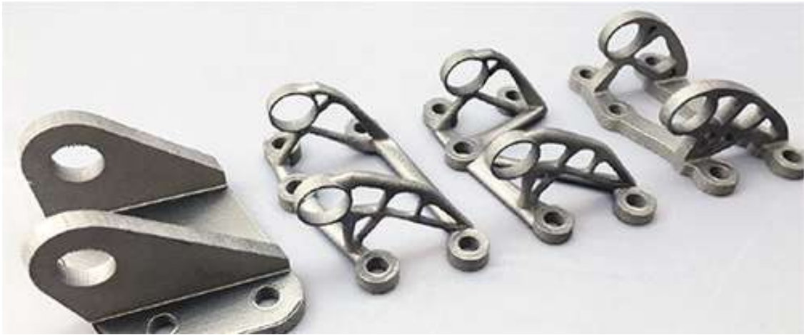
Figure 1.16: Aerospace bracket produced with SLM technology after topological optimization [52].
