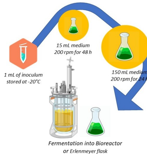
Figure 4-1 Propagation procedure for A. vinelandii fermentation. In the image, the standard procedure of A. vinelandii cultivation is reported from the inoculum of a glycerol stock stored at -20°C to the final cultivation set in a bioreactor or flask.
