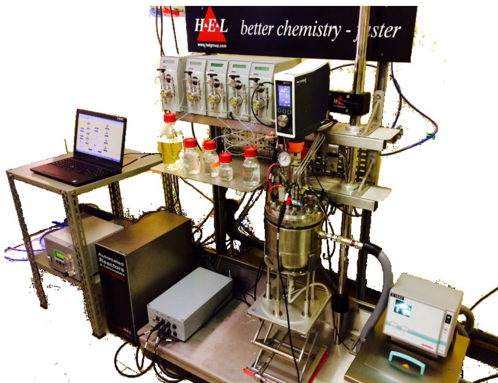
Figure 3-2 2L pressurized bioreactor designed for overpressure reactions and used during the experimentation.
