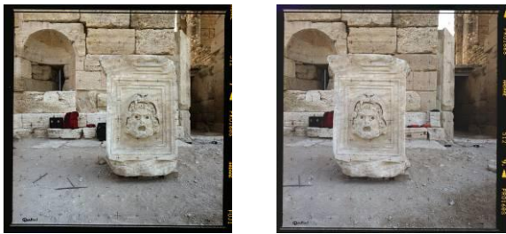
Figure 11 A stereoscopic acquisition of a theatrical mask using the Rollei 6006
