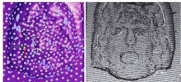
Figure 5 STL 3D model and target acquired during a scan (left), point clouds visualizartion (right)
