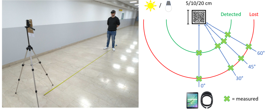
Fig. 1. Setting for DD/LD/DR/ST with artificial light using the HoloLens™ (left) and experimental setup for DD/LD (right)
