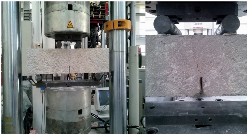
Figure 6 – Four-point bending test, notched specimen.
