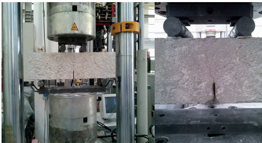
Figure 6 – Four-point bending test, notched specimen.
