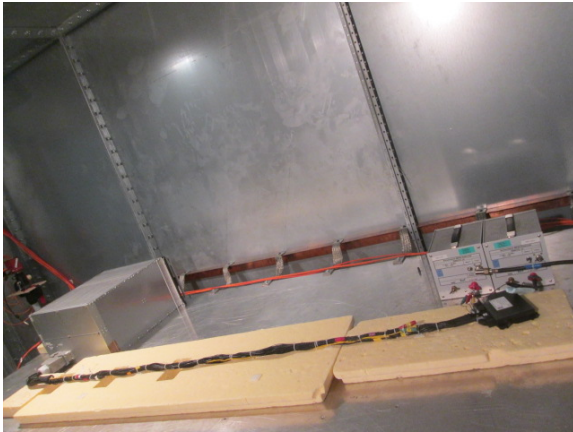
Fig. 2 Conducted emissions setup in shielded room
