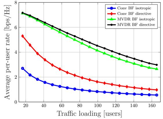
Fig. 2: Average per-user rate as a function of the network load (average number of users in  $\mathcal{B}$ ). Comparison for a UCylA with isotropic and directive antennas, implementing conventional and MVDR BF.  $N_c=90$ ,  $N_z=4$
