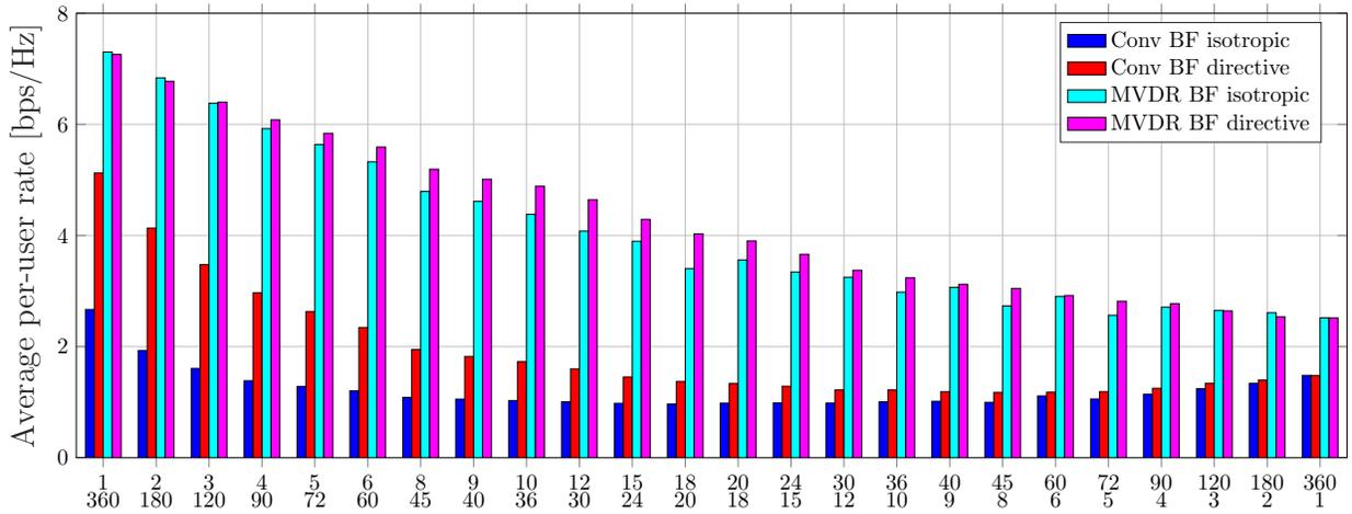
Fig. 3: Average per-user rate in UCylA for different number of rings  $N_c$  and antennas along z-axis  $N_z$  with both isotropic and directive elements implementing conventional and MVDR BF with  $N = N_c \cdot N_z = 360$ . For  $N_c = 1$ ,  $N_z = 360$ , antennas are only isotropic.  $M = 60$  users.
