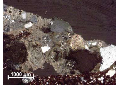
Fig. 13. Bedding mortar of the bricks of the frames, characterized by a fat mixture (image at the optical microscope in thin section, polarised light), (Rescic).
