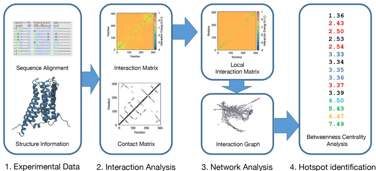
**Fig. 1.** Schematic representation of the workflow. We employ available sequence alignments and structures to build a coevolution-based interaction matrix that we refine using a contact map, building a network that contains spatial and interaction information about the protein of interest. Hotspots are finally identified by means of the analysis of the betweenness centrality of every node, that are subsequently labeled based on the data available in the literature.
