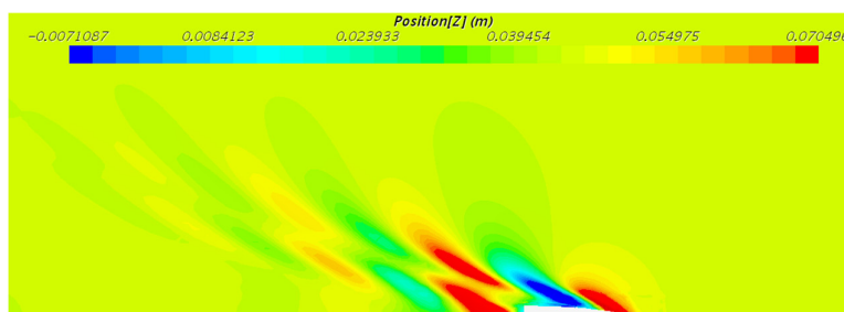
Figure 9. Wave pattern behind the hull for 3 m/s.
