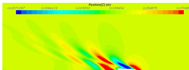
Figure 9. Wave pattern behind the hull for 3 m/s.
