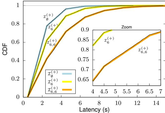
Figure 6: Measured and theoretical CDFs of  $d$  (channel hopping disabled).
