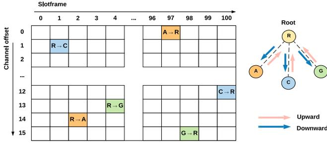
Figure 1: Sample TSCH Matrix (3 downward and 3 upward cells).
