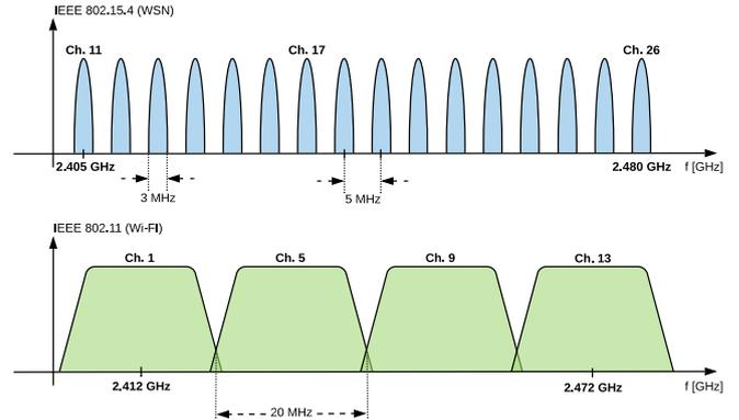
Figure 4: Overlapping channels in IEEE 802.11 and 802.15.4 (ISM band).
