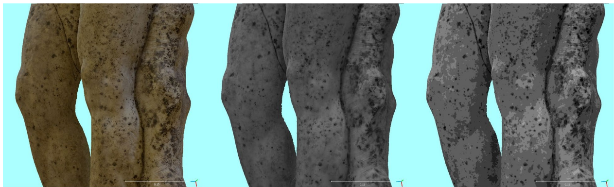
Fig. 4 Marble statue, close-up comparison between visible (left), near-infrared (center) textures and 8-group classification mapping of near-infrared intensities (right)
