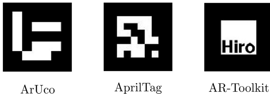
Figure 1. Examples of square fiducial markers.
