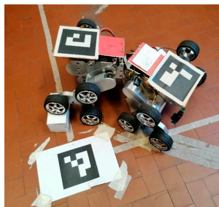
Figure 7. Epi.q mod2, the remotely controlled mobile robot used for testing the localization system with moving markers while climbing a little obstacle. The markers with ID 1 and 2 are fixed respectively on the front (left in the photo) and rear (right) module. The fixed reference (Marker ID 0) is fixed to the floor instead.
