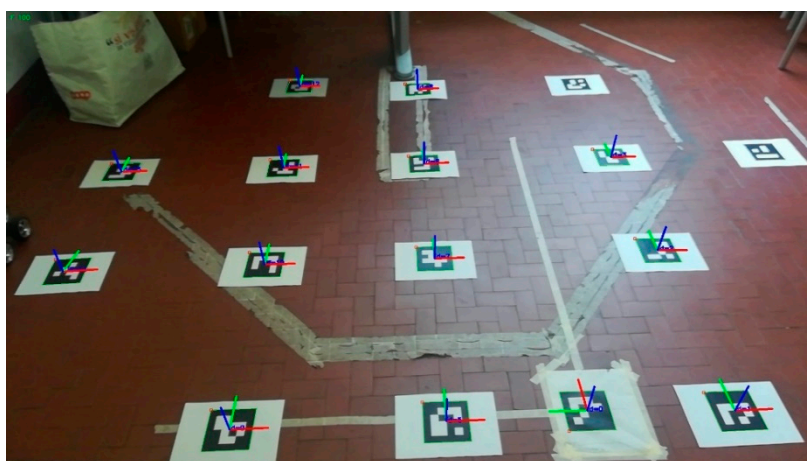
Figure 6. Setup to evaluate the static performance of the system. This picture also shows that the algorithm places a reference frame at each identified marker center, while the unidentified ones remain without axes.
