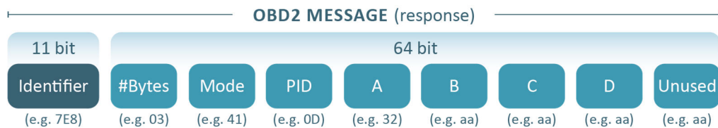
Figure 34. Typical structure of an OBD response message (source: www.csselectronics.com )
