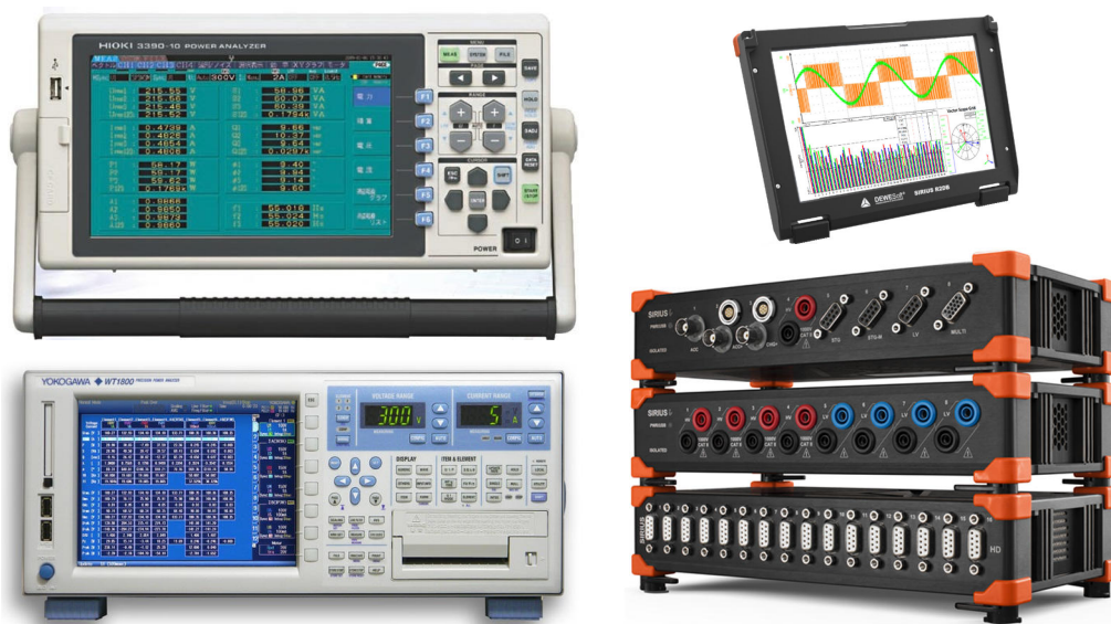
Figure 36. Power analysers of the JRC-STU (Hioki top left, Yokogawa bottom left, Dewesoft right)
