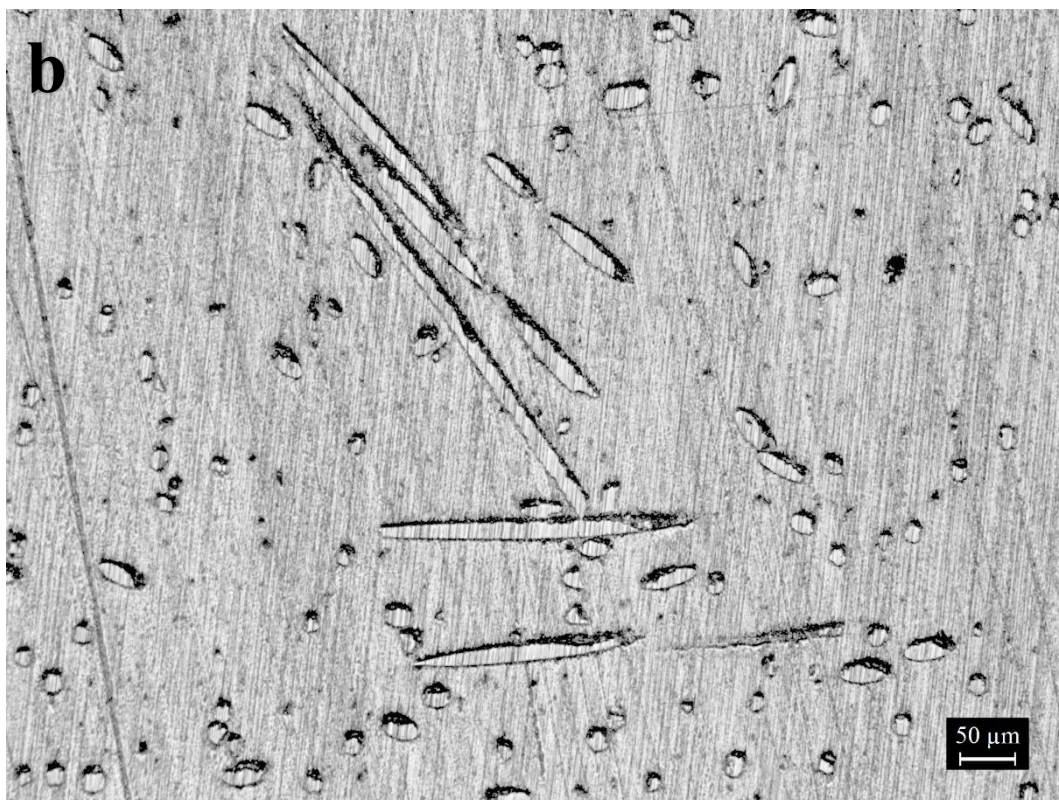
Figure 6.6 Optical micrographs of the section of the CM-PA6-15GF composite at different magnification (a) 50X, (b) 100X.
