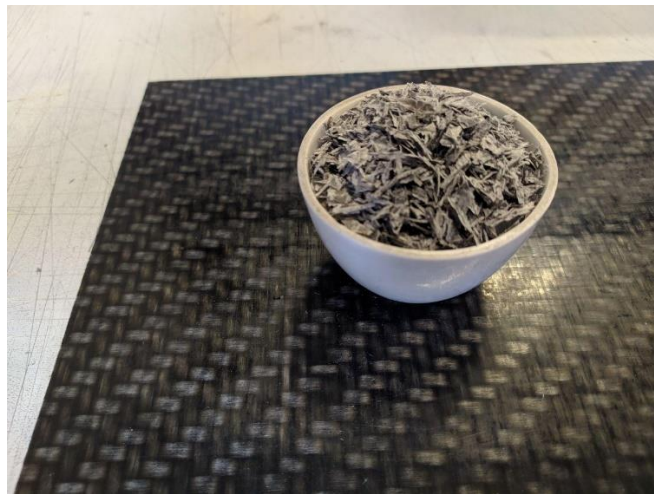
Figure 4.3 Laminate made of polyamide 6 reinforced with 47% roving glass fibers before and after grinding.
