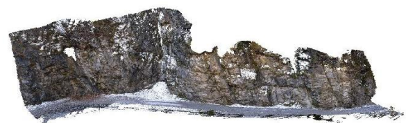
Figure 7. Example of "vertical" terrestrial dense point cloud.
