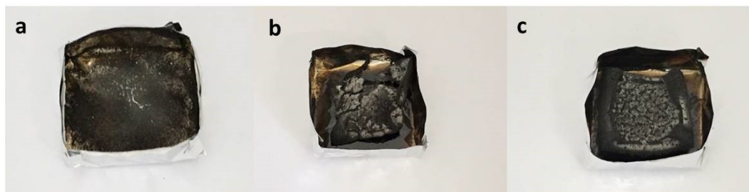
Figure 42 Images of a) untreated PU foam, b) 3 BL and c) 6 BL foams cone calorimeter residue.
