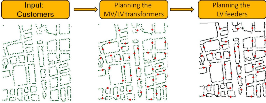
Figure 3.5: Identification of customer and MV/LV substation positioning
