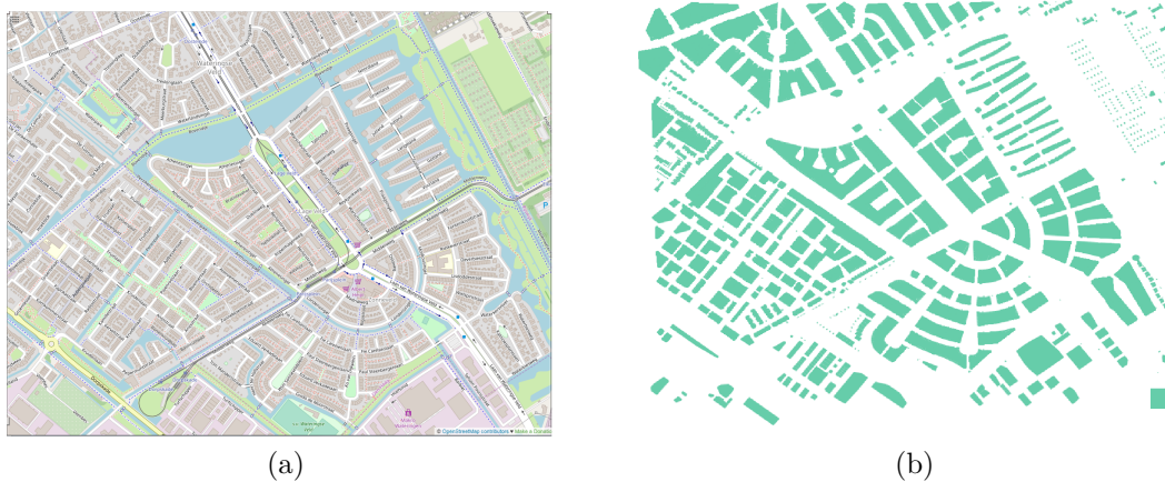
Figure 4.11: OpenStreetMap image of The Hague in (a) and building detection in (b)
